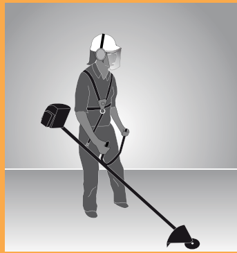
FIGURE 28: The heaviest part of this brush cutter is located behind the wrists and the weight is supported by a harness.
