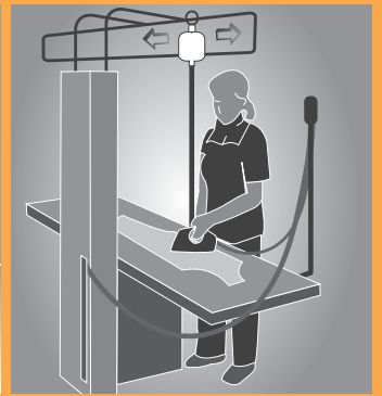
FIGURE 28: An overhead suspension system reduces the forces required to use the iron.
